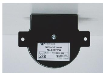
**Step 4:** Screw on the two side screws, and plug in the power of the dome.
