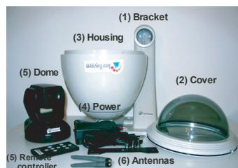
**Step 1:** Get the power wire through the bracket first.
